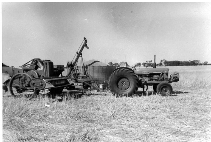
Harvest 1960-61. Fordson Tractor and 8ft McKay header and auger. Field bin lined with hessian
